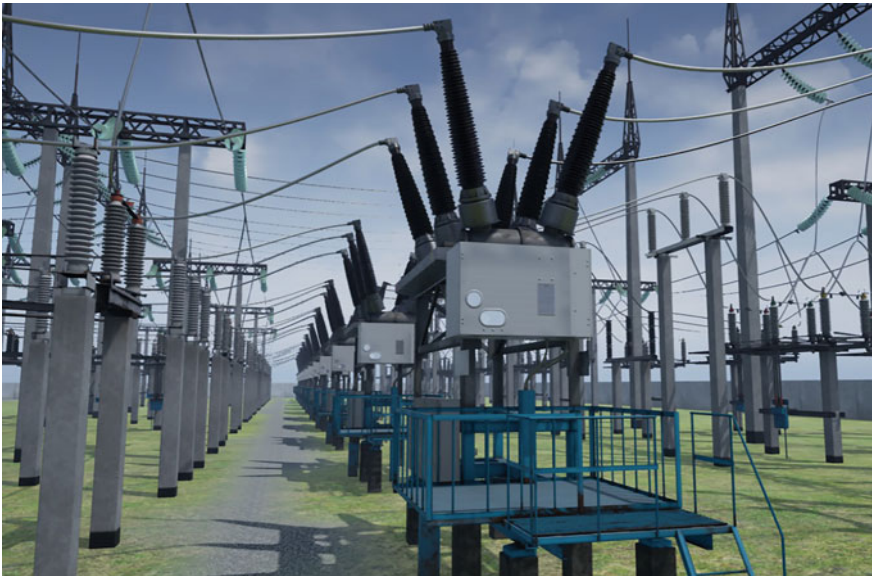
Fig. 19.6 3-D model of a 110 kV sulfur hexafluoride circuit-breaker
