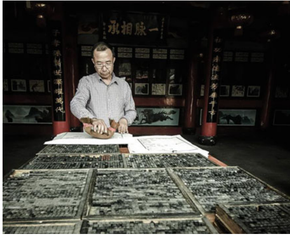
Fig. 5.11 Brush pressing by a local craftsman onto wooden movable printing type in the Rui'an area of Zhejiang Province
