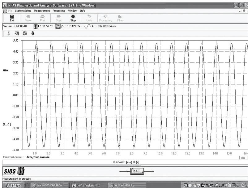
FIGURE 13.10 Demonstration of open loop repeatability of a PZT flexure.
