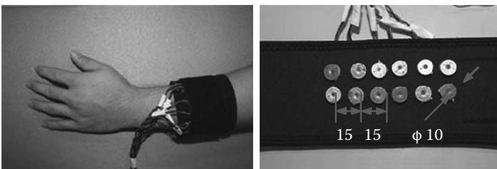
FIGURE 12.2 Multichannel sEMG sensor ring: (a) sensor ring on the forearm and (b) six-channel sEMG electrodes.
