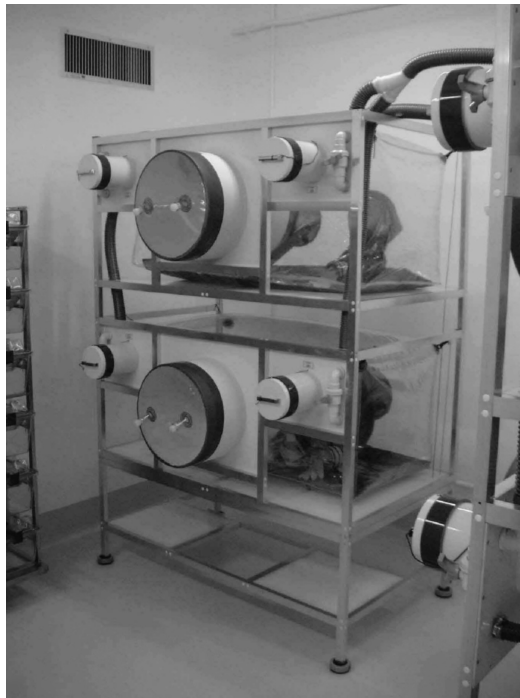
FIGURE 3.7 Flexible film isolator for rodents, an example. (Photo courtesy of T. P. Rooymans.)
