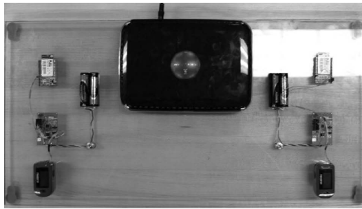
Figure 25.12 Wearable pulse oximeter for telemedicine with Wi-Fi link.
