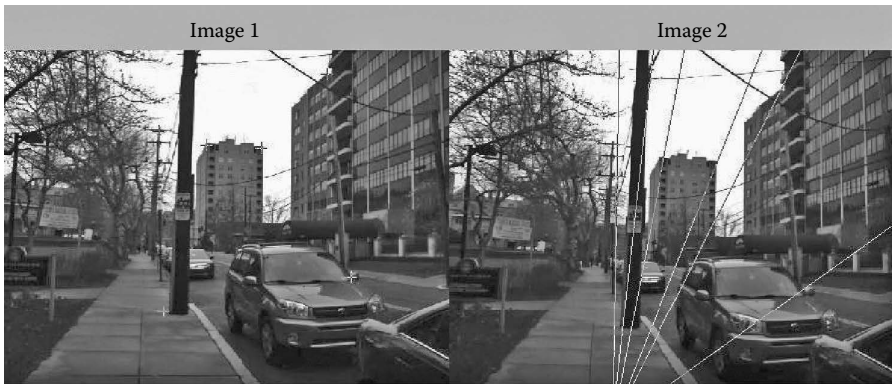
FIGURE 9.13 (See color insert.) Feature points in Image 1 versus Epipolar lines in Image 2.
