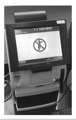
Figure 6.5 Blood gas analyzer.
