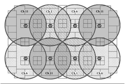
Figure 3.1 A 2.4-GHz channel plan.
