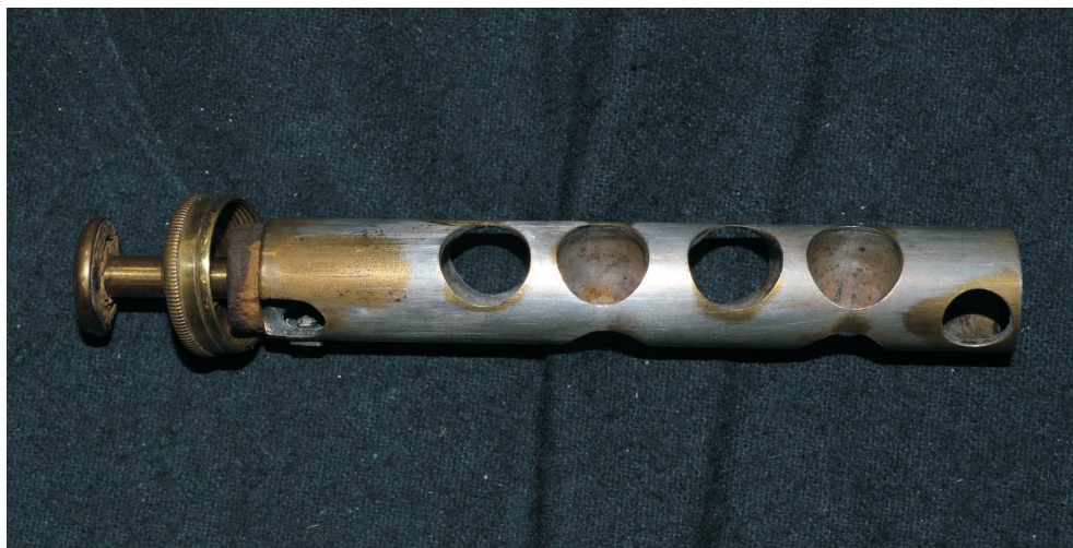
FIGURE 3 Dual airflow valve, cor Sax à 6 pistons, serial number 37403, Brussels MIM inventory number 3167. Photo: Jeroen Billiet by courtesy of MIM Brussels
