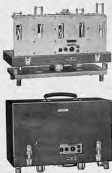
The Tapping Machine Type 3202 is designed as a standardized noise generator of impact sound for use in measurements of impact sound insulation in buildings. It is made in accordance with the specifications given in "Provisional Code for Field and Laboratory Measurements of Airborne and Impact Sound Insulation". The brass hammer heads are interchangeable by heads of hard wood, whereby is obtained that the Tapping Machine meets the requirements of the previous type of impact sound generator.
