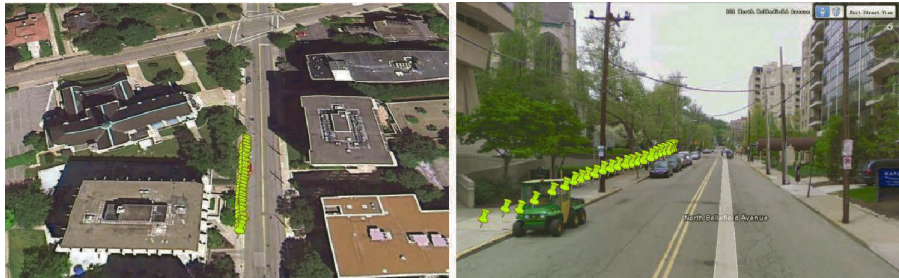
FIGURE 9.14 Positioning results by using visual odometry, top view (left) and street view (right).
