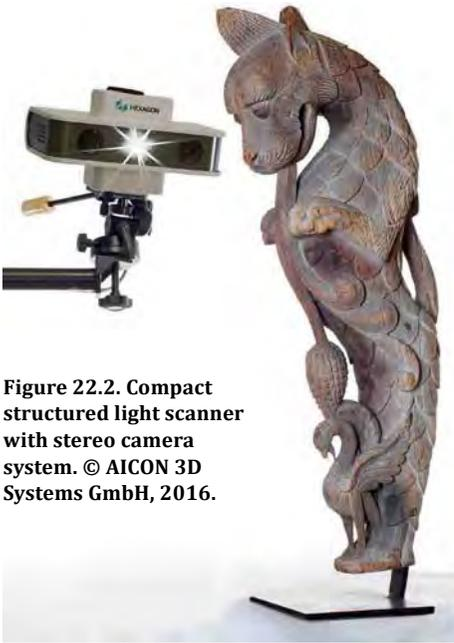
**Figure 22.2.** Compact structured light scanner with stereo camera system. © AICON 3D Systems GmbH, 2016.
