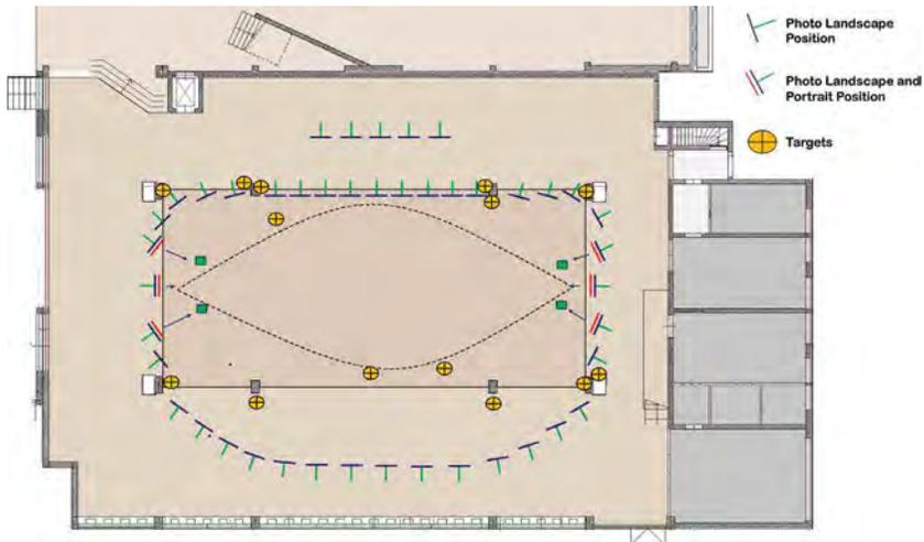
**Figure 7.3. Bremen Cog floor plan, common coordinate system on the ground floor.**
