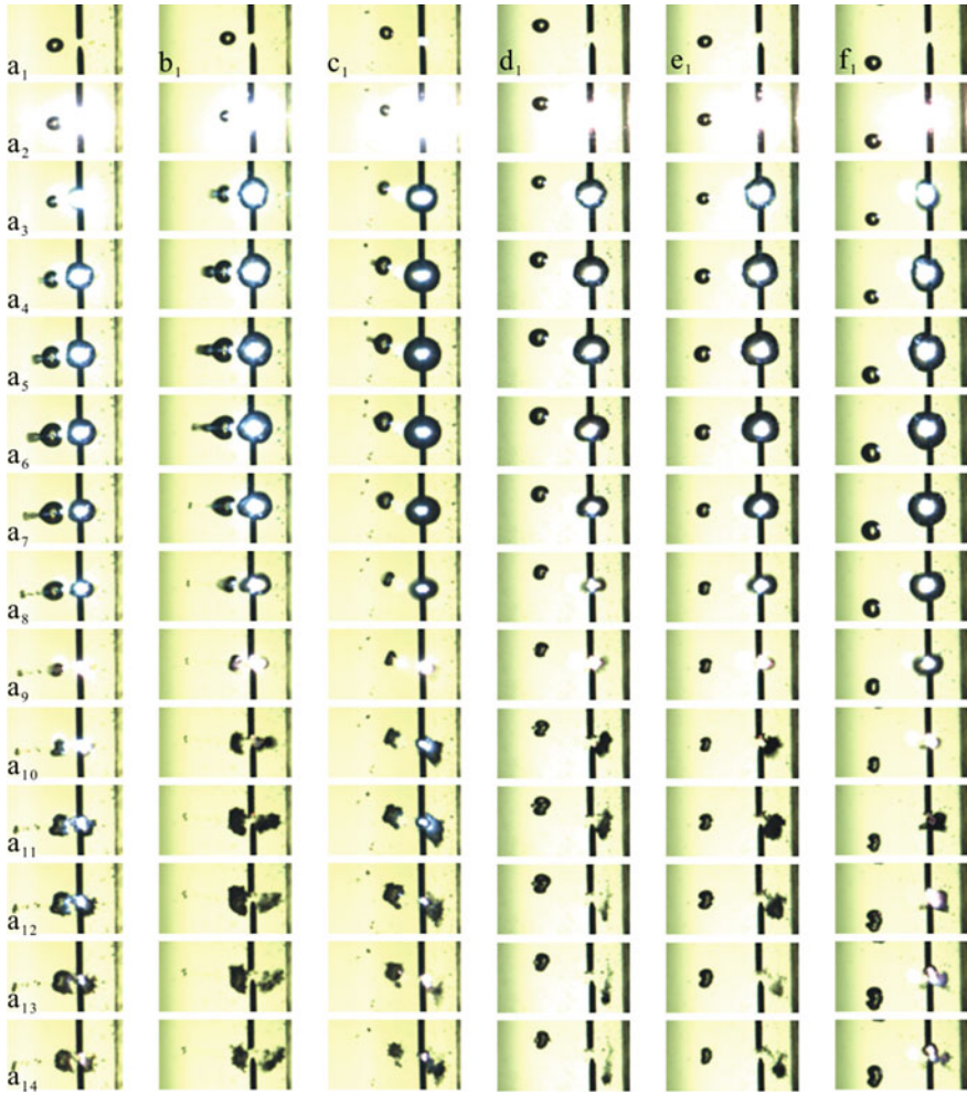
Fig. 3.28 Air bubble-cavitation bubble-wall interaction at the same value of \gamma and different values of \omega (frame rate: 19,700 fps; exposure time: 48 us; image size: a 12.133 * 7.367 mm; b-f 13.867 * 7.367 mm; the spatial relationship between the air bubble, cavitation bubble, and wall is shown in Table 3.2)
