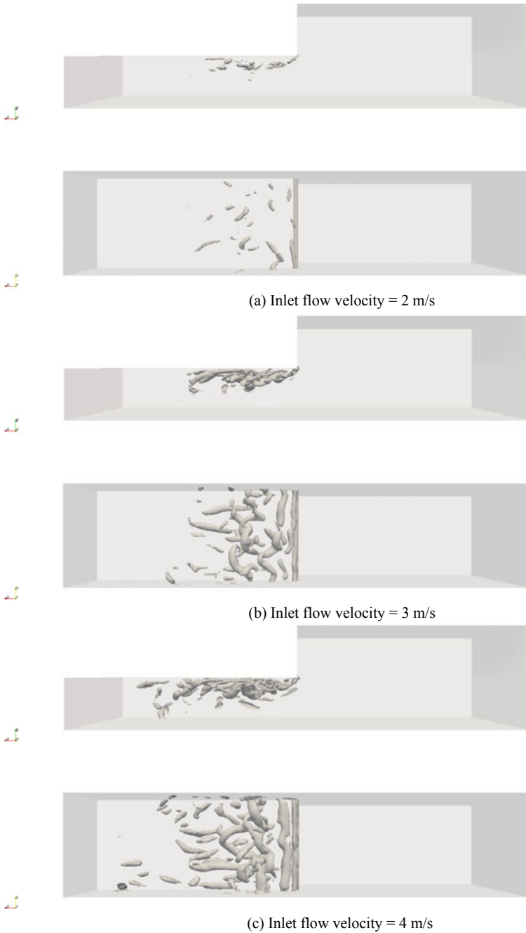
Fig. 5.12 Vortex blob at different flow velocities (contour surface \lambda_2 = -50000 )
