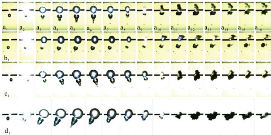
Fig. 3.32 Cavitation bubble-air bubble-wall interaction at different cavitation bubble-wall distances ( 90^\circ < \theta < 270^\circ ; frame rate: 19,700 fps; exposure time: 48 us; image size: a 13.867 * 7.367 mm; b 13.867 * 7.367 mm; c 17.333 * 7.367 mm; d 17.333 * 7.367 mm; the air bubble-cavitation bubble-wall spatial relationship is shown in Table 3.6)
