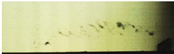
Fig. 2.29 CB formed when contraction ratio \beta = 0.799 and mean inflow velocity u_0 = 7 m/s
