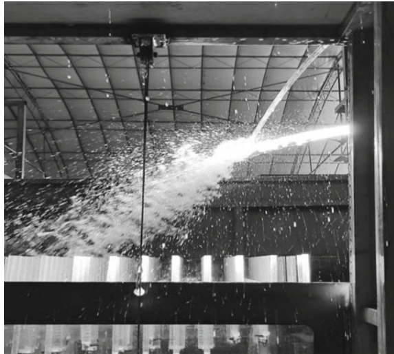
Fig. 6.24 Water droplets formed from spallation of jets as a result of collision in air
