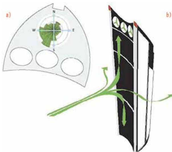
Figure 5. Orientation study based on prevailing wind direction; site plan sketch with wind rose (a) and an illustration of airflow distribution around the tower (b) © BFLS.
