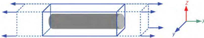
Figure 3.16: Longitudinal deformation of a simulation box.
