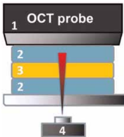
Figure 5. Schematic of OCT imaging setup: 1 is the OCT scanner ( \lambda = 1.3 \mu\text{m} ); 2 is the soft silicone layer; 3 is the studied biopolymer sample (e.g., samples of cartilaginous or corneal tissues); 4 is the source of the heating infrared irradiation (erbium fiber laser operating at \lambda = 1.56 \mu\text{m} ).
