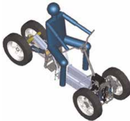
Figure 2. The diagram of narrow tilting vehicle in RESOLVE Project developed by AIT [6].
