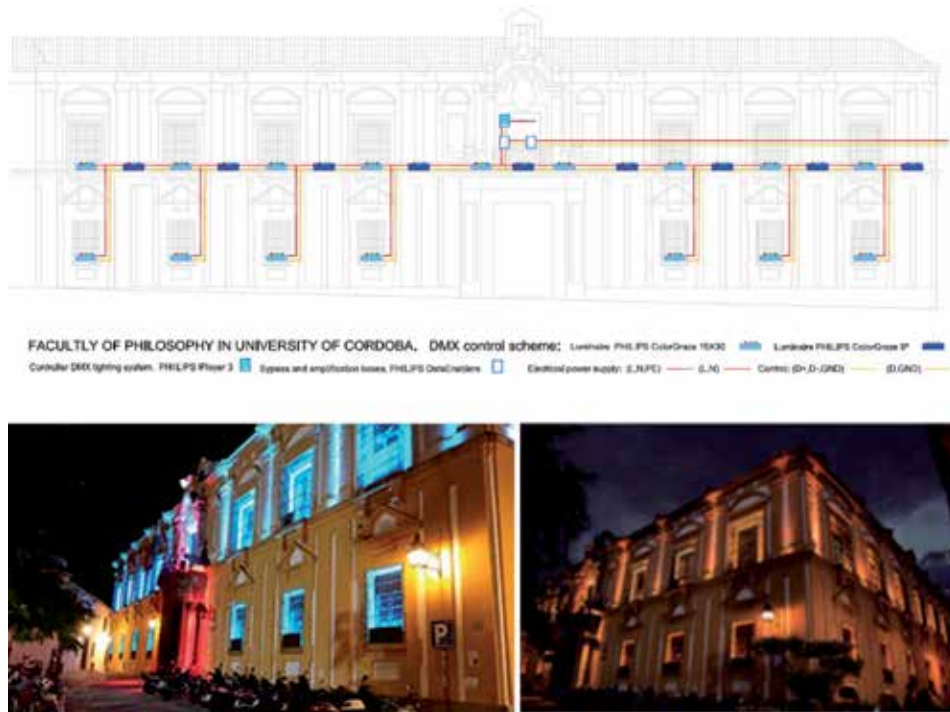
Figure 4. Lighting and sound show Faculty of Philosophy in University of Córdoba, year 2017. Linear installation scheme formed by Color Grace luminaires of 9° and 15 × 30°, three DataEnablers, iPlayer controller, and wiring between supply (L,N) and data (D,GND) luminaires. As a temporary installation, a bypass box was not placed. Source: own elaboration.
