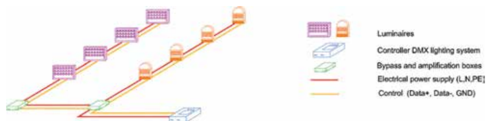
Figure 3. Diagram of the DMX control scheme principles. Source: own elaboration.
