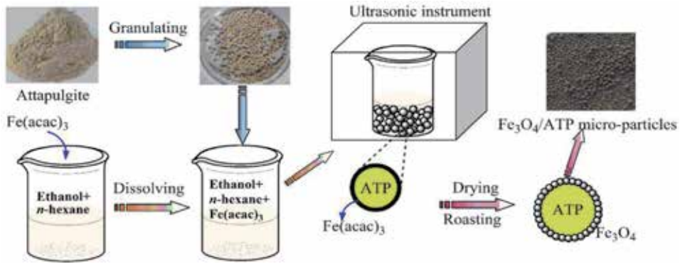
Figure 11. Schematic of preparing Fe 3 O 4 /ATP catalyst [24].
