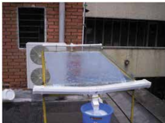
Figure 9. Pilot-scale solar flat plate reactor used for degradation of a model pollutant.
