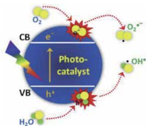
Figure 19. Photocatalytic process in semiconductor.
