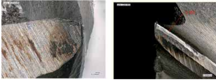
Figure 8. Notch wear and flank wear ( V_c = 30 m/min, emulsion-based nanofluid) at 40 min [16].
