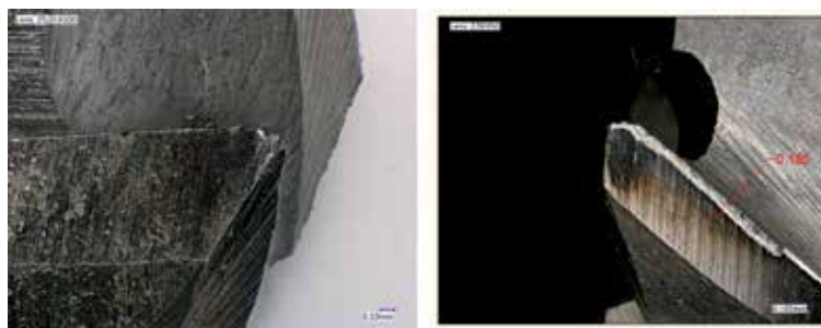
Figure 7. Notch wear and flank wear ( V_c = 24 m/min, emulsion-based nanofluid) [16].
