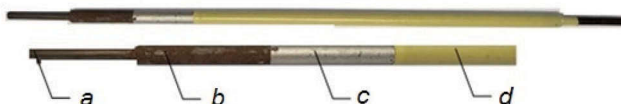
Figure 1. The structure of the Arcair Sea-Weld electrode; a – electrode core wire, b – iron oxide layer, c – aluminum covering, d – plasticized vinyl.
