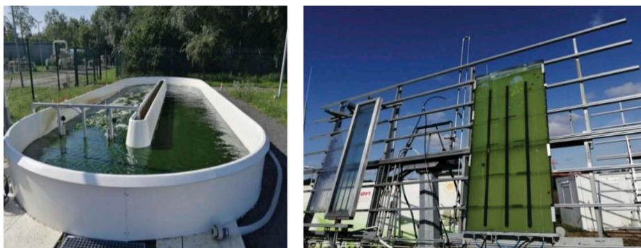
Figure 1. Types of cultivation systems (outdoor conditions): a – open raceway pond; b – closed photobioreactor.
