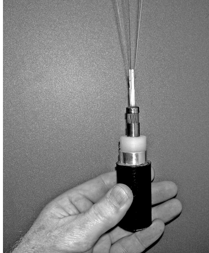
Figure 23.2 A section of lightweight cable designed for deployment on the seabed surface, nominally in water depths exceeding 2000 m, which is the approximate depth limit of deep trawl fishing, a major cause of cable faults
