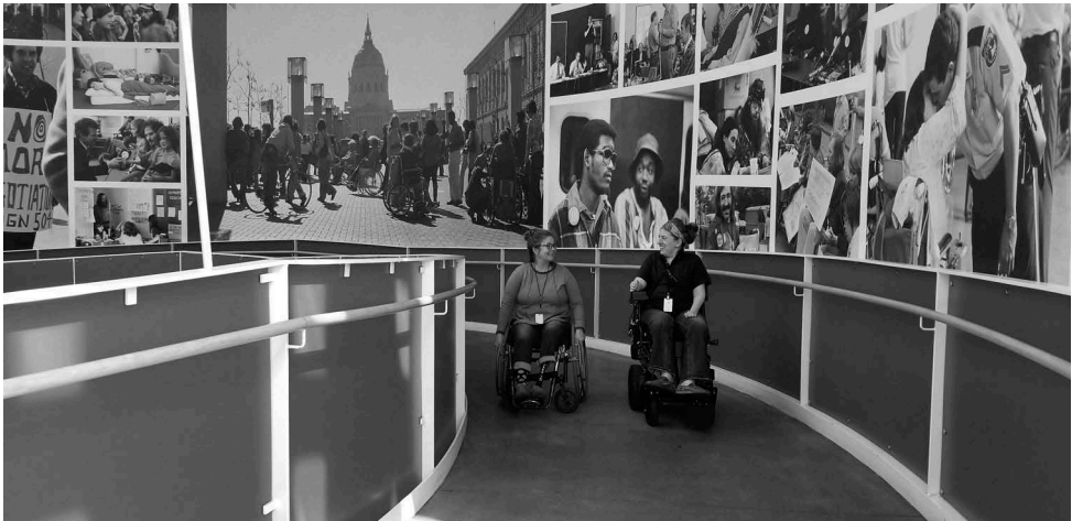
FIGURE 5.1 Large central ramp that easily fits two wheelchair riders side by side and that was integrated into the design of Patient No More in the lobby of the Ed Roberts Campus. Photograph by Fran Osborne.
