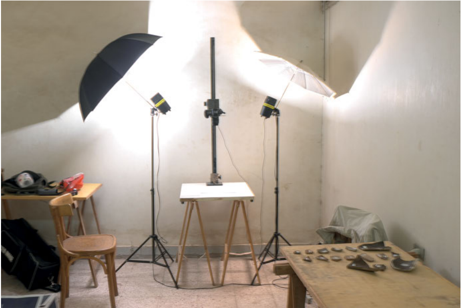
Fig. 3: Typical set-up when photographing ostraca in the storeroom in Egypt: A copy-stand and two flashes with umbrellas, to give even, diffused light. If you are photographing papyri under glass, you will need to remove the umbrellas and turn the flashes directly onto the reproduction-surface, since the umbrellas will almost certainly make reflections in the glass. Here the lights are set at a higher angle than 45^\circ (c. 70^\circ ) since there is no risk of reflections.
