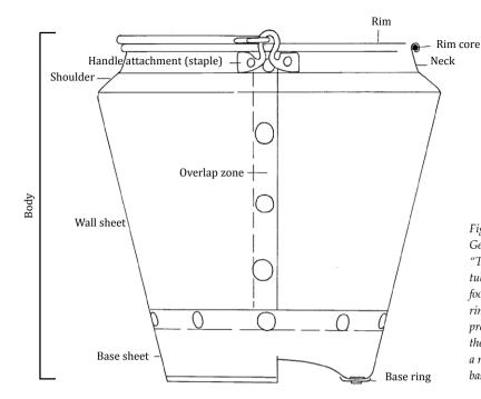
Fig. C2.2 Bucket terminology (adapted from Gerloff 2010, 41–3; Prüssing 1991, abb. 1). "The bottom sheet of the vessel is formed into a tub shape. The base of the tub is formed into a flat foot ring surrounding a hollow omphalos. The foot ring and its angle with the side of the vessel are protected by a variety of strengthening devices, the base- or angle plates. If these are in the form of a ring-shaped single casting, this is referred to as base ring" (Gerloff 2010, 41–3).
