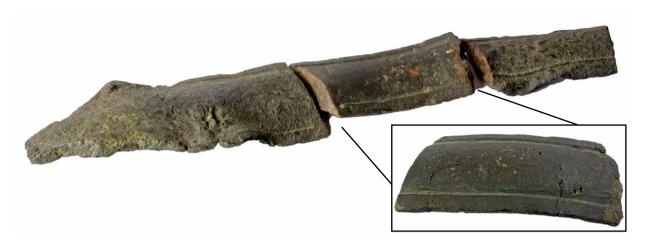
Fig. C6.32 The three surviving fragments of a bronze sword (CSE-LQ.UC.23; the tang is on the left) with detail of the middle fragment (reverse side) showing cracks in the bronze (inset). Photographs by J. van Donkersgoed.
