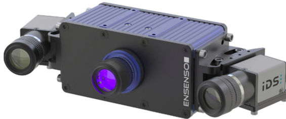
Fig. 4. Stereo camera system offered by Ensenso GmbH [4].
