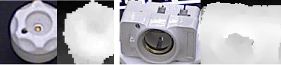
Fig. 5. RGB and depth images of the objects 2 and 6 from the T-LESS dataset, respectively. Many of the small cues are not observable in the depth modality while easily observable in RGB.
