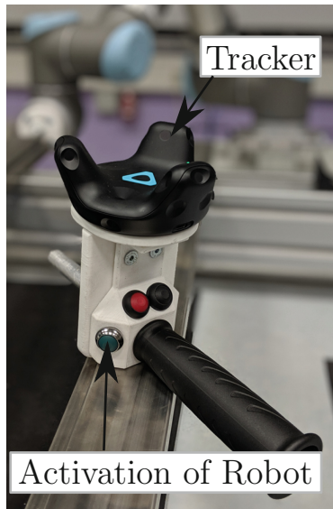
Fig. 3. Worker tool with tracker.
