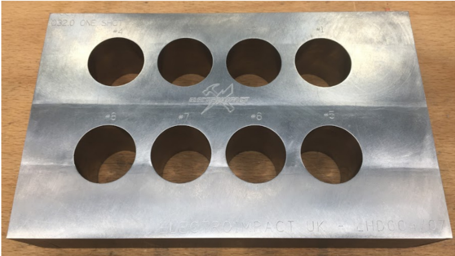
Fig. 5. 32.0 mm test coupon a (guehring tipped drill)
