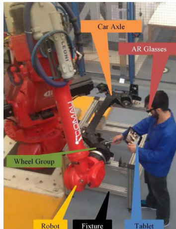
Fig. 17. Application of a see-through AR system to assist an operator in a cooperative work with a robot (source: [32]).
