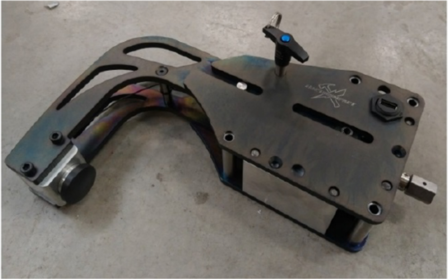
Fig. 17. Manual panel clamp with load cell feedback
