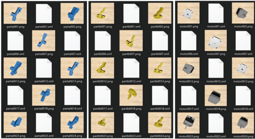
Fig. 2.13 Generated 2D image dataset from the virtual 3D virtual model of the assembly
