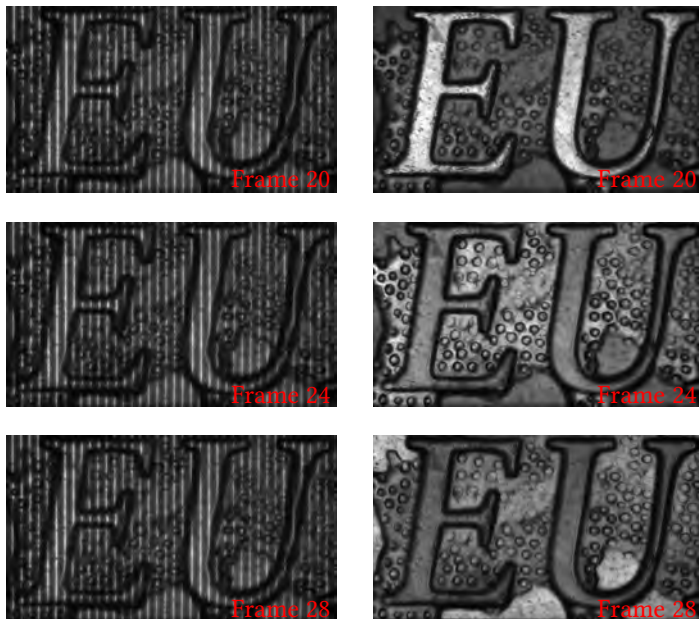
Figure 5.18: Left column: raw camera frames from direct area scanning. Right column: confocal signal through reordering of the raw signal.
