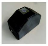
**Figure 2.1:** Handheld *SmartSpectrometer* device based on the NeoSpectra Micro development Kit. To determine the degree of maturity, the reflection spectrum is recorded non-destructively and evaluated directly in the embedded device.
