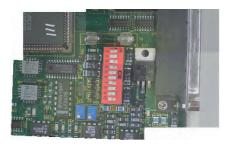
**Figure 1.3:** Not optimal stitching result.
