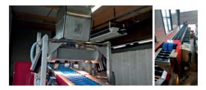
Figure 2.3: Infeed to the Sherlock Food Analyzer with Conveyor System and Ejection Unit.
