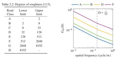
Figure 2.3: Power spectral density of road profiles.
