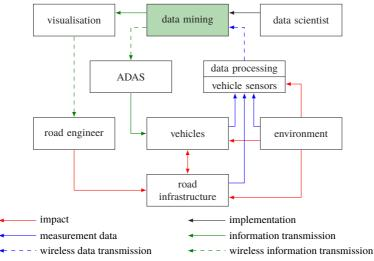
Figure 3.1: Overview of the data flow and participants of a novel concept for road condition monitoring with on-board vehicle sensors.
