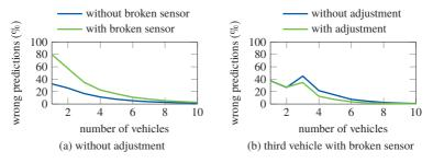
Figure 6.21: Results of vehicle combination: Scenario 3. Classification with and without broken sensor. a: 1st vehicle with and without broken sensor. b: 3rd vehicle with broken sensor with and without automated adjusting precision matrix for this vehicle.
