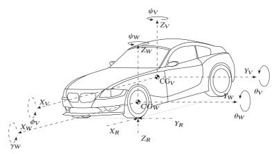
Figure 2.1: Vehicle with three translational and three rotational degrees of freedom. The reference point of the vehicle axis system  $X_V$ ,  $Y_V$ ,  $Z_V$  with the angles  $\psi_V$ ,  $\phi_V$ , and  $\theta_V$  is placed in the center of gravity of the vehicle (CG<sub>V</sub>). One of four wheel axis systems  $X_{W4}$ ,  $Y_{W4}$ ,  $Z_{W4}$  is defined with the angles  $\theta_{W4}$ ,  $\psi_{W4}$ ,  $\gamma_{W4}$ .
