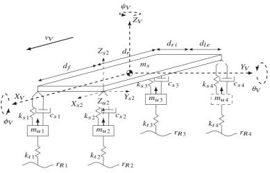
Figure 3.11: Full car model for vertical dynamics simulation.
