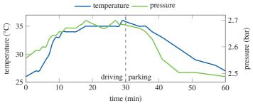
Figure 3.9: Tire temperature and pressure acquired with TPMS.
