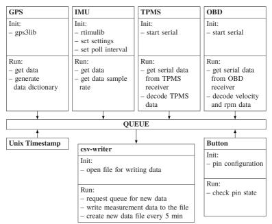
Figure 5.3: Structure of the main da ta collection service *sensorrecorder.py* with processing tasks for each sensor as separate, independent threads. The data is combined and tagged with a timestamp in a csv-table.
