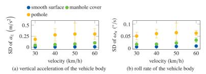
Figure 4.6: Vehicle vibration (standard deviation (SD)) due to road features for various velocities.
