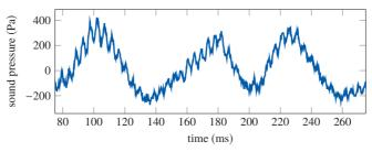
Figure 3.6: Time series of tire cavity sound.
