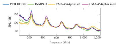
Figure 6.3: SPL with a 1/12 octave band smoothing of all microphones during vehicle operation with constant speed of 60 km/h.
