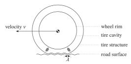
Figure 3.3: Vibration of the tire due to road irregularities.
