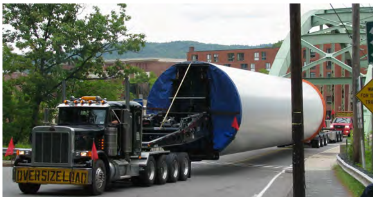
Figure 2.10: Tower section transport under the 1935 Ramford bridge [116]
