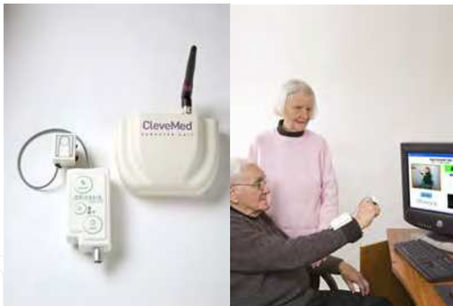
Fig. 1. Kinesia, Cleveland Medical Devices Inc. system for PD monitoring based on motor sensors (Jovanov et al., 2001)
