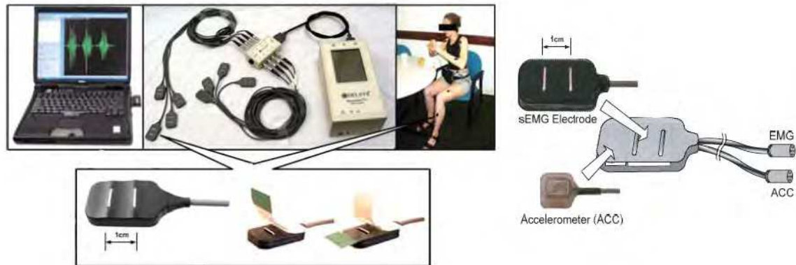
Fig. 8. Boston University National Institute of Biomedical Imaging and Bioengineering, PD monitoring system through motor and EMG sensors (UB, 2011)
