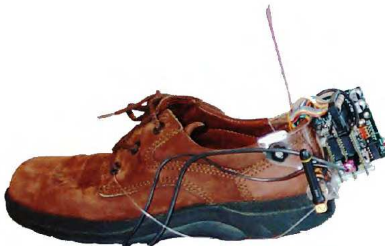
Fig. 5. Sensor Shoe, University of Twente, Enschede, The Netherlands. Gait analysis based on movement sensors (Kauw-A-Tjoe et al., 2007)
