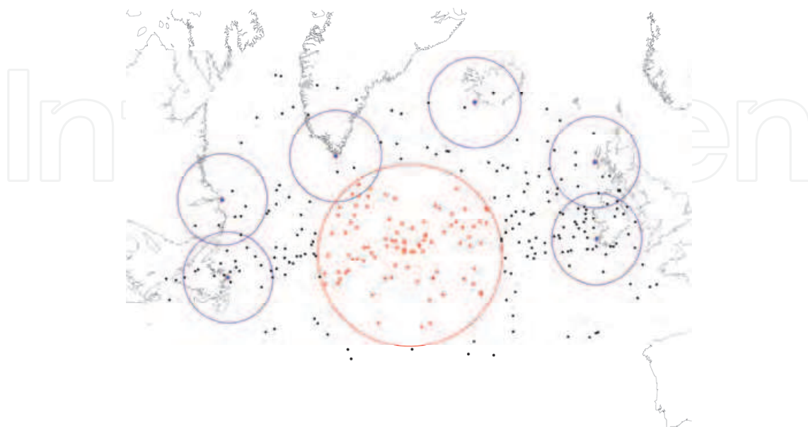
Fig. 5. Air-to-air (red) and air-to-ground (blue) LOS range at FL350.
