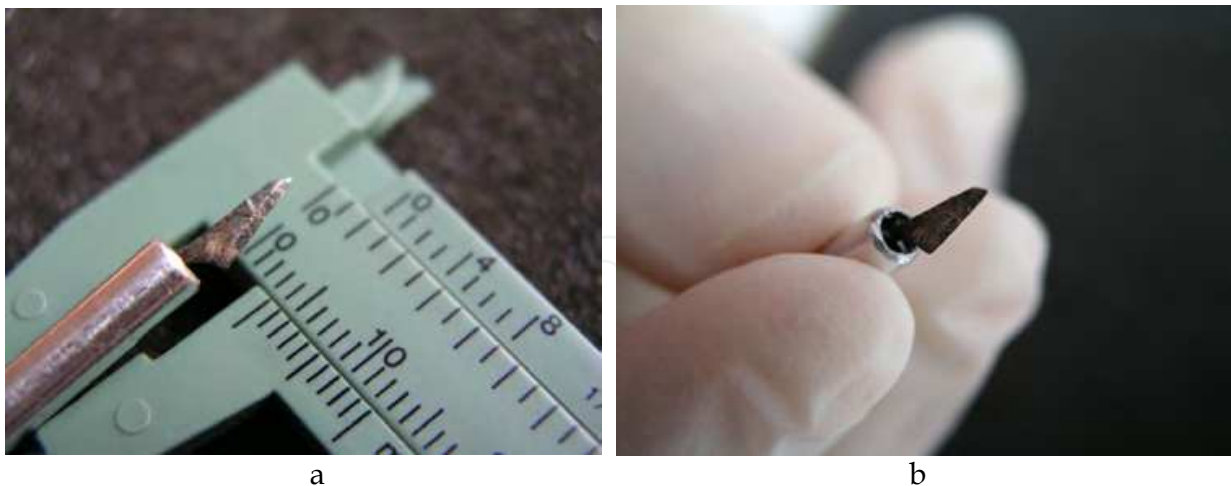
Fig. 6. Final prototype has an outer diameter of 4 mm
