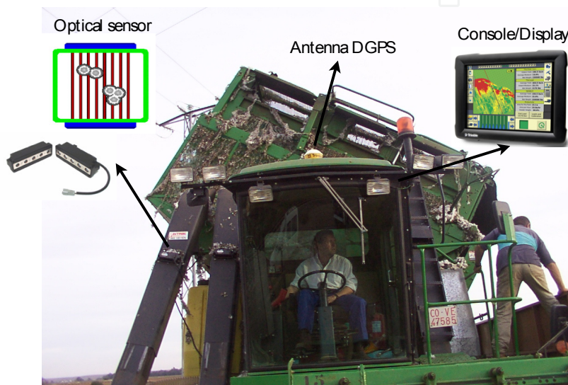
Figure 6. Cotton yield monitor mounted and used at University of Cordoba, Spain. The combine is equipped with 4 optical flow sensors, a DGPS receiver and a display.
