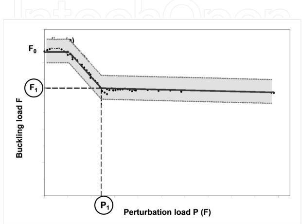
Figure 4. Scatter of buckling load due to the scatter of non-traditional imperfections
