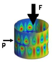
Figure 2. Perturbation load mechanism
