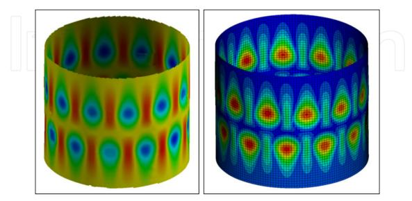
Figure 13. Postbuckling pattern. Left: Test results obtained by ARAMIS - Right: Simulation results
