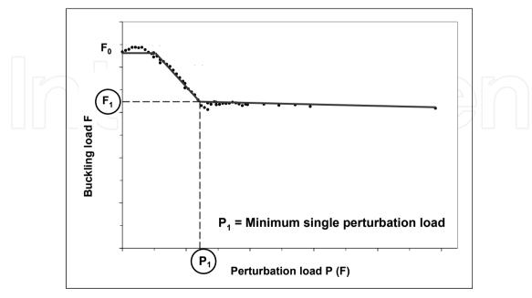
Figure 3. Single perturbation load approach (SPLA)
