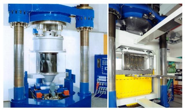
**Figure 7.** DLR's buckling test facility, axial compression configuration (left), compression-shear-configuration (right)
