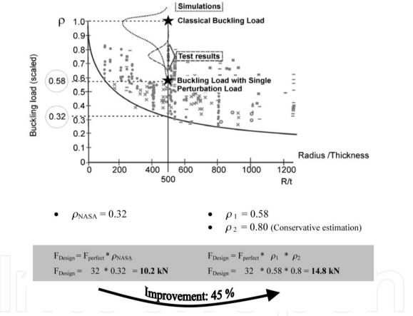
**Figure 6.** Potential of the future design scenario [2] Example: CFRP cylindrical shell (R/t = 500, 4 layers), F<sub>perfect</sub> = 32 kN
