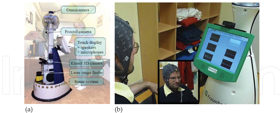
Figure 11. The ALIAS robot utilizes several different sensors to perceive the user's input and intentions (a). In addition, it supports BCI systems through the intendiX ACTOR protocol and by embedding visual stimuli and feedback modalities using the intendiX SOCI module (b).
