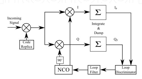
Figure 1. Carrier phase tracking loop
