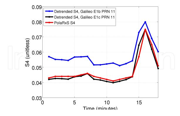
**Figure 5.** Comparison of  $S_4$  values obtained by the Septentrio PolaRxS receiver and estimated values of Galileo E1b/c PRN 11 obtained by the software receiver.
