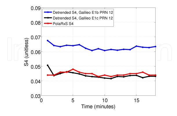
**Figure 4.** Comparison of  $S_4$  values obtained by the Septentrio PolaRxS receiver and estimated values of Galileo E1b/c PRN 12 obtained by the software receiver.
