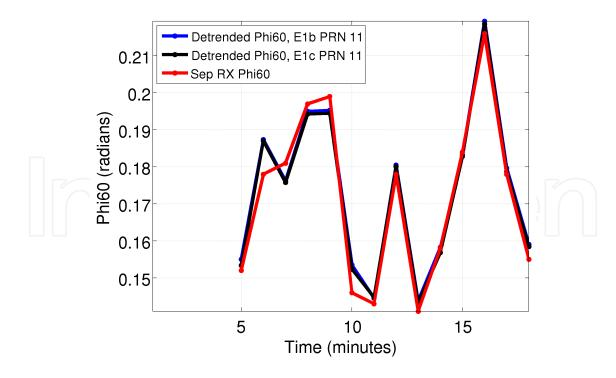
**Figure 7.** Comparison of Phi60 index obtained by the Septentrio PolaRxS receiver and the estimated values of Galileo E1b/c PRN 11 obtained by the software receiver. Small deviations in Phi60 are due to temporal misalignment between the estimated and the Septentrio values.
