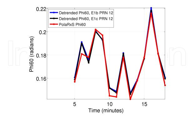
**Figure 6.** Comparison of Phi60 index obtained by the Septentrio PolaRxS receiver and estimated values of Galileo E1b/c PRN 12 obtained by the software receiver. Small deviations in Phi60 are due to temporal misalignment between the estimated and the Septentrio receiver values.
