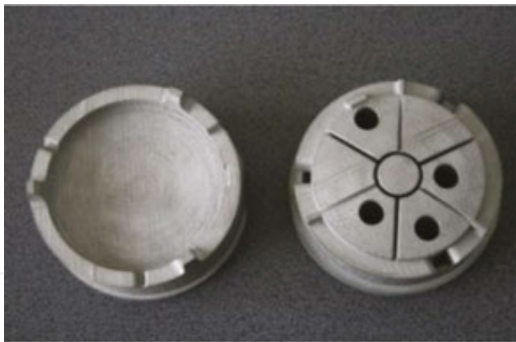
Figure 7. The injection moulding tools made by SLM equipment.
