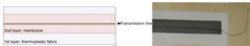
Figure 15. Schematic diagram and real photo of a hot air welded transmission line.
