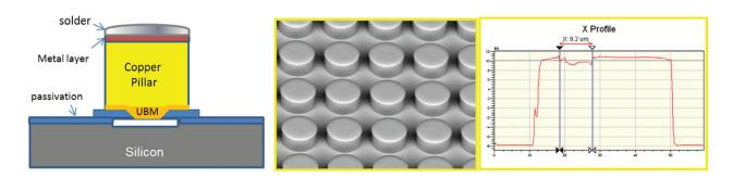
**Figure 14.** Images of copper pillars and lead-free micro-bumps at 50  $\mu$ m pitch. The profile shows the pillar bump after probing with vertical MEMS probe technology.
