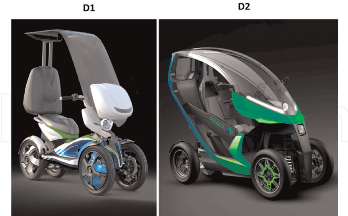
Figure 1. Two demonstrators of narrow tilting vehicle developed in the RESOLVE Project [8].
