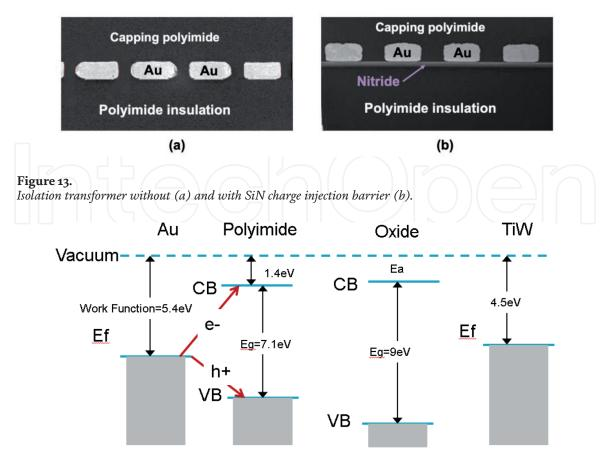
**Figure 14.** Band diagram for charge injection.
