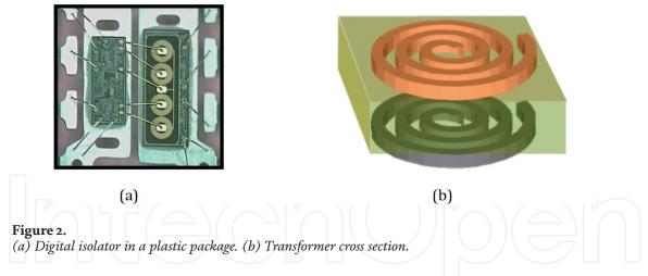
less than 2.5 pF capacitance between the input and output. Because of these characteristics, polyimide is increasingly used in microelectronics applications, and it is an excellent choice as insulating material for the *i*Coupler high voltage digital isolators.
