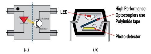
**Figure 1.** (*a*) Opto-coupler schematic. (*b*) Opto-coupler package cross section.
