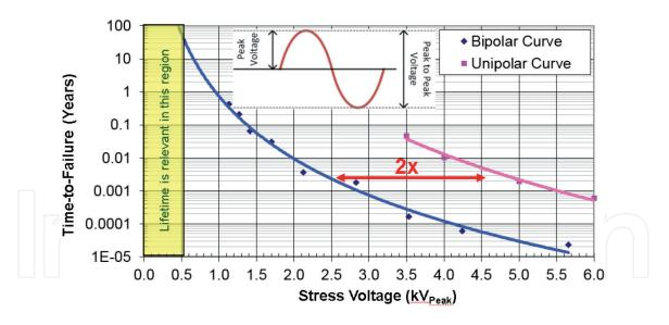
**Figure 12.** *Time-to-failure comparisons for AC bipolar versus unipolar.*
