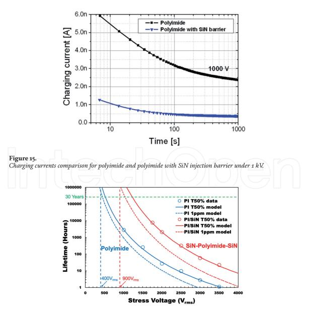
**Figure 16.** *Time-to-failure comparison for polyimide isolators with and without SiN charge injection barrier.*
