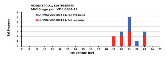
**Figure 7.** Surge performance for isolators with polyimide films 30 µm thick.
