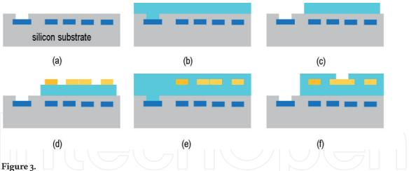
Isolation transformer process flow. (a) CMOS substrate with top metal, (b) polyimide layer spin coated, (c) polyimide layer patterned  $\mathfrak{G}$  cured, (d) top coil plated, (e)  $2^{nd}$  polyimide layer spin coated and (f)  $2^{nd}$  polyimide layer patterned  $\mathfrak{G}$  cured.
