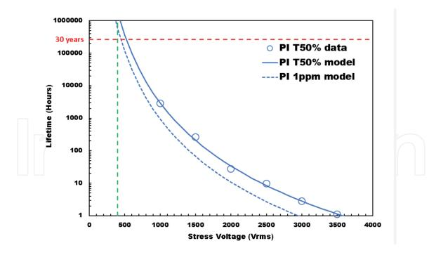
**Figure 10.** *Time-to-failure plot for isolators with 20-µm thick polyimide.*
