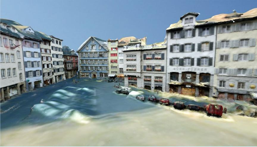
2. RÉSULTAT INTERMÉDIAIRE DU MODÈLE 3D. IL MONTRÉ UNE APPROCHE STANDARD POUR CRÉER ET TEXTURER DES MODÈLES DE SURFACE. VARCITY VA PLUS LOIN ET ANALYSE CE QUI EST VISIBLE, TOUT COMME UN ÊTRE HUMAIN COMPRENDRAIT CETTE VUE DE MÜNSTERHOF, ZÜRICH (ERC VARCITY PROJECT @ COMPUTER VISION LAB, ETH ZÜRICH).
