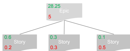
Fig. 5.4 Proportions of the epic's benefit points and story points distributed on stories.
