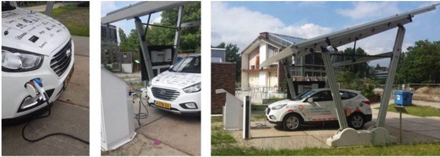
Fig. 6 The Europe's first Vehicle-to-grid connection using hydrogen fuel cell electric vehicle and the local electricity grid at The Green Village, Delft University of Technology
