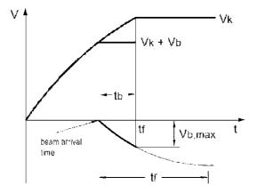
Fig. 8.25. Conceptual diagram illustrating multi-bunch,  $\Delta t$  beam loading and energy compensation
