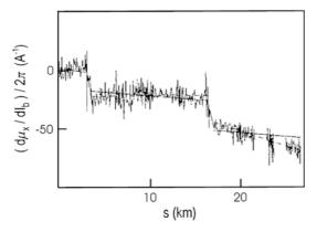
Fig. 2.10. Dependence of the horizontal betatron phase advance on the bunch current,  $d\phi/dI_b/(2\pi)$  in units of A<sup>-1</sup>, measured at LEP [23] (Courtesy A. Hofmann, 1998)
