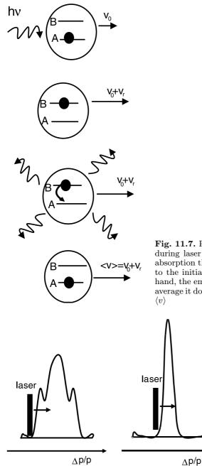
Fig. 11.7. Photon absorption and emission during laser cooling [5]. After each photon absorption the recoil component  $v_r$  is added to the initial ion velocity  $v_0$ . On the other hand, the emission is isotropic and, thus, on average it does not alter the final ion velocity  $\langle v \rangle$
