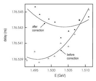
Fig. 7.10.  $R_{56}$  measurement for the asynchronous arc of the KEKB linac, before and after dispersion correction. A streak camera was used to measure the arrival time (*vertical axis*) as a function of the beam energy (Courtesy H. Koiso and K. Oide, 1998)
