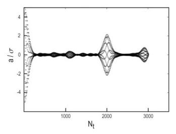
Fig. 11.13. Simulated centroid position in units of  $\sigma$  as a function of turn number for a normalized detuning  $\mu = -2 \times 10^{-4}$  [49]. A first kick of  $5\sigma$  applied at turn 0 is followed by second kick of strength  $0.25\sigma$  at turn 1000. A clear echo signal is seen around turn 2000, and a second echo at turn 3000
