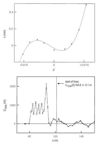
Fig. 7.5. Evidence of 3rd order dispersion in the SLC ring-to-linac transfer line (RTL) [14]: (top) Horizontal beam position versus beam energy; (bottom) 3rd order dispersion inferred for all BPMs in the RTL and in the early linac. The 3rd order dispersion in the linac is fitted to calculate the magnitude of the  $U_{1666}$  and  $U_{2666}$  matrix elements (Courtesy P. Emma, 1998)
