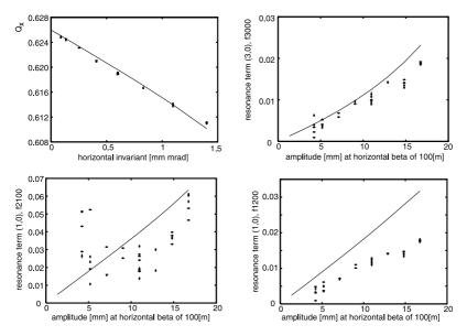
Fig. 2.27. Detuning and first-order resonance driving terms, measured at the SPS [60]. Shown are the betatron tune  $[top \ left]$  and the relative amplitude of several resonance lines with respect to the main tune line [other] as a function of the oscillation amplitude. Plotting symbols are experimental data; lines are from a tracking simulation. 170 turns were sampled per point (Courtesy F. Schmidt, 2000)
