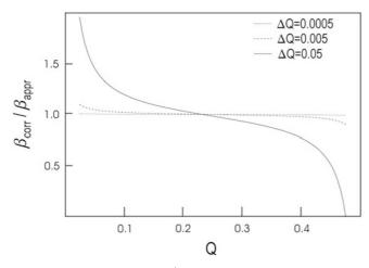
Fig. 2.11. The ratio  $\beta_{\text{corr}}/\beta_{\text{appr}}$  of the correct beta function  $\beta_{\text{corr}}$ , inferred from (2.28), to the approximation  $\beta_{\text{appr}}$  given in (2.29) as a function of the nominal tune Q. The three curves correspond to different magnitudes of  $\Delta Q$
