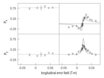
**Fig. 10.10.** Demonstration from the IUCF of polarization preservation in the vicinity of an imperfection resonance using a 10% partial siberian snake (*left*) and loss of polarization without the partial snake (*right*). In these measurements the kinetic energy of the beam was fixed at 105.9 MeV
