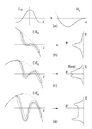
Fig. 8.19. Conceptual illustration for optimizing the relative phase of the beam for the case of very long bunches. The accelerating field  $E_{\rm rf}$  and the longitudinal wake field  $W_{\parallel}$  are shown in (a). The longitudinal profiles and their projections onto the energy axes are shown for different relative phases (between the beam and the rf wave) in (b)–(d) (Courtesy J. Seeman, 1999)
