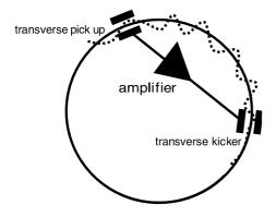
Fig. 11.6. Schematic of stochastic cooling
