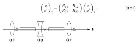
**Fig. 3.12.** Simple FODO lattice. Shown are the focussing quadrupoles (QF), the defocussing quadrupoles (QD), and dipoles (rectangles). The BPMs are usually mounted within the quadrupoles. Corrector magnets are denoted by triangles
