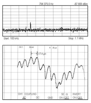
Fig. 2.29. Monitoring betatron coupling at the ATF Damping Ring [71]. (top) Frequency spectrum of a horizontal pick up on a spectrum analyzer; (bottom) evolution of the peak signal in the frequency spectrum as a function of time, as viewed on an oscilloscope; the slow variation reflects synchrotron motion, the fast beating with a period of about 17.6  $\mu$ s is due to the transverse coupling; the amplitude and period of the modulation can be used to determine the driving term  $|\kappa_-|$
