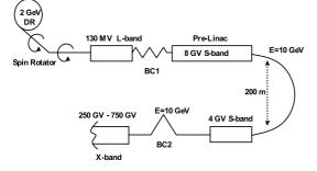
Fig. 8.1. Schematic of an NLC bunch compressor [6]
