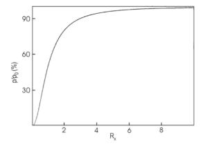
Fig. 2.16. Systematic slope error introduced in a linear  $\chi^2$  fit of the form y = px+q, neglecting the noise smearing in the x measurement [33]. Shown is the reconstructed slope normalized to the true slope as function of signal-to-noise ratio  $R_x$  in the horizontal coordinate (Courtesy P. Emma, 1998)
