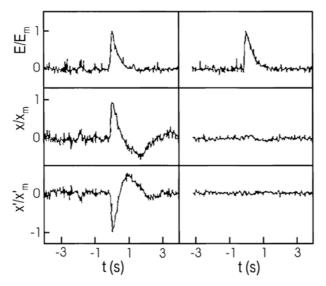
Fig. 3.21. Response of the orbit and energy feedback in the ring-to-linac transfer line of the SLC to a fast step change in energy [43]: (*left*) before and (*right*) after additional BPMs were included in the feedback loop
