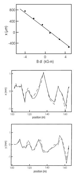
Fig. 3.13. Example of an  $R_{12}$  measurement: transverse position x versus  $\int B \, dl$ , where the kick angle, in terms of the magnetic rigidity  $B\rho$ , is  $\theta = \int B \, dl/(B\rho)$
