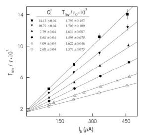
Fig. 2.21. Coherent damping rate in LEP as function of bunch current measured at a beam energy of 45.625 GeV for several chromaticities Q' [54]. The *straight lines* are fits to the individual samples. The *table* gives measured chromaticities and 'zero current' damping rates (Courtesy A.-S. Müller, 2001)
