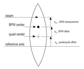
Fig. 3.1. Sketch showing relative positions of the BPM, the quadrupole, and the beam position measurement from an ideal reference axis (Courtesy C. Adolphsen, 1999)
