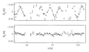
Fig. 7.3. Vertical dispersion measured via a  $\pm 5 \text{ kHz}$  rf frequency ramp at the KEK ATF Damping Ring before [top] and after correction [bottom] [6]; a dispersion of  $D_y = 5 \text{ mm}$  corresponded to an orbit change of  $\Delta x \approx 15 \text{ }\mu\text{m}$  (Courtesy J. Urakawa, 2000)
