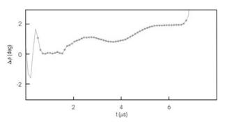
Fig. 8.24. Measured phase difference between the PEP-II electron (HER) and positron (LER) beams (Courtesy P. Corredoura, 2000)
