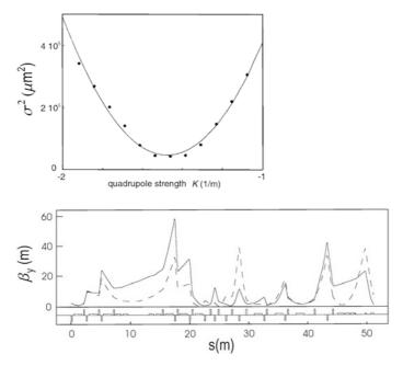
**Fig. 4.11.** Beta matching in the KEK/ATF beam transport line (BT) [11]: (*top*) quadrupole-scan emittance measurement; shown is the square of the vertical beam size measured using a fluorescent screen vs. the strength of an upstream quadrupole; (*bottom*) the vertical beta function obtained by propagating the measured Twiss parameters (*solid*) through the actual BT optics is compared with the beta function expected for the design optics (*dashed*)
