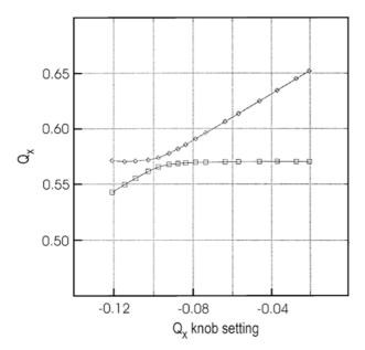
Fig. 2.30. Closest tune approach in the PEP-II HER before final correction [73]. Shown are the measured fractional tunes as a function of the horizontal tune 'knob' (which would only change  $Q_x$  if the accelerator were uncoupled), in dimensionless units. The minimum tune distance is equal to the driving term  $|\kappa_{-}|$  of the difference resonance (Courtesy Y. Cai, 1998)
