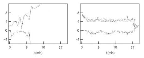
Fig. 7.15. Variation of chromaticity in time, due to persistent-current decay without (*left*) and with (*right*) chromaticity control based on continuous measurements of the sextupole fields in two dipole reference magnets at the HERA proton ring [25]. The horizontal axis is the time in units of 3 minutes per division. The vertical axis refers to the horizontal (*upper trace*) and vertical chromaticity (*lower trace*) in dimensionless units (Courtesy B. Holzer, 1998)
