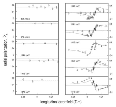
Fig. 10.7. Measurements of time-averaged radial polarization at the IUCF near a  $G\gamma = 2$  imperfection resonance (at about 106.4 GeV) at 5 different beam kinetic energies with a 100% siberian snake on (*left*) and off (*right*)
