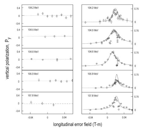
Fig. 10.8. Measurements of time-averaged vertical polarization at the IUCF near a  $G\gamma = 2$  imperfection resonance (at about 106.4 GeV) at 5 different beam kinetic energies with a 100% siberian snake on (*left*) and off (*right*)
