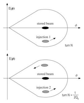
Fig. 9.5. Double injection into the same rf bucket; bunches are injected off-energy at a point with dispersion [8]. Time between the two injections is half a synchrotron oscillation period modulo a full period (Courtesy P. Baudrenghien and P. Collier, 2001)
