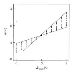
Fig. 3.6. Beam-based alignment of a single quadrupole at the TTF (Courtesy P. Castro, 2000)
