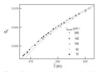
**Fig. 7.7.** Synchrotron tune  $Q_s$  as a function of total rf voltage in LEP; the two curves are fits to the 640  $\mu$ A and 10  $\mu$ A data. The difference due to current-dependent parasitic mode losses is clearly visible. Here the nominal beam energy  $E_{\text{nom}}$  was 60.589 GeV [15] (Courtesy A.-S. Müller, 2000)
