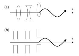
Fig. 3.3. Conceptual drawing illustrating orbit perturbations due to misaligned quadrupoles (a) or structures (b)
