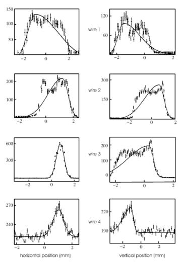
Fig. 4.4. Raw data showing individual wire scans used in the summary display of Fig. 4.3 and the "asymmetric Gaussian" fits of (4.37)
