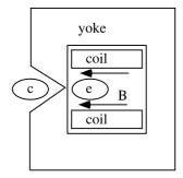
Fig. 9.14. Schematic of Lambertson septum iron magnet [2]; the symbol c represents the circulating beam, the symbol e the extracted beam
