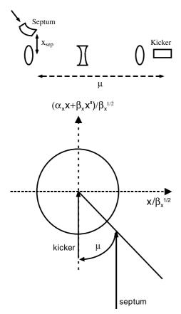
Fig. 9.1. Schematic of single-turn injection with septum and kicker: (top) magnet arrangement, (bottom) phase-space diagram. The septum strength is adjusted to place the beam onto the line describing an angle  $\mu$  (the phase advance from septum to kicker) with respect to the vertical [1]
