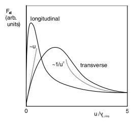
Fig. 11.4. Cooling force  $F_{\rm el} = Mu/\tau_{\rm el}$  in a flattened electron beam as a function of ion velocity u in units of the rms electron velocity in the beam frame  $v_{e,\rm rms}$ . The *dashed curve* corresponds to the asymptotic formulae derived in the text. The difference between the transverse and longitudinal plane is due to the temperature difference, which arises from the longitudinal acceleration. Picture is redrawn from [5]
