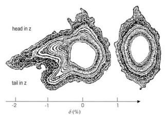
Fig. 8.17. Measurements of the beam profile at a dispersive location at low compressor voltage (*left*) and with bunch overcompression (*right*) (Courtesy F.J. Decker, 2000)
