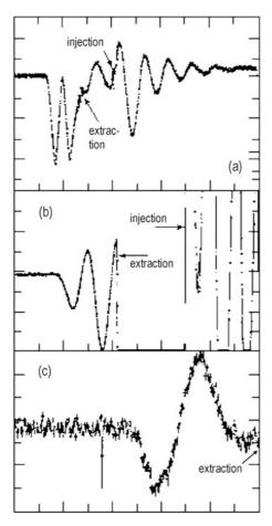
Fig. 8.2. Bunch precompression in the SLC damping rings: (a) measured cavity voltage [50 kV/dvsn, 10  $\mu$ s/dvsn], (b) peak current [10%/dvsn, 5  $\mu$ s/dvsn], and (c) centroid energy [50  $\mu$ m or 0.77%/dvsn, 20 turns or 2.34  $\mu$ s/dvsn]
