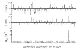
**Fig. 3.2.** Typical commissioning orbit in the PEP-II HER: (top) horizontal orbit in mm; (center) vertical orbit in mm; (bottom) intensity in  $10^{10}$  (Courtesy U. Wienands, J. Seeman *et al*, 1998)
