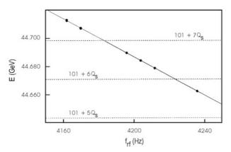
**Fig. 7.11.** Change of beam energy E as a function of the rf frequency  $f_{\rm rf}$  in LEP [19]. Only the last four digits of the rf frequency are shown (the nominal value is  $f_{\rm rf} = 352\ 254\ 170\ {\rm Hz}$ ). Several strong spin resonances are indicated by the dotted lines. From this measurement the momentum compaction factor was determined to be  $(1.86\pm0.02)\times10^{-4}$ , which compared well with the calculated value of  $1.859\times10^{-4}$  (Courtesy R. Assmann, 1998)
