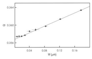
**Fig. 2.24.** Tune as a function of Courant-Snyder invariant with the 108/90 degree phase advance optics at an arc monitor in LEP [54]. The *straight line* is a fit to the data (Courtesy A.-S. Müller, 2001)
