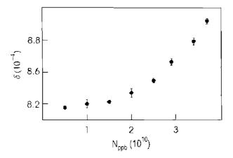
Fig. 8.14. Measured energy spread of beams exiting the SLAC electron damping ring as a function of beam current. The total cavity voltage in this measurement was 945 kV
