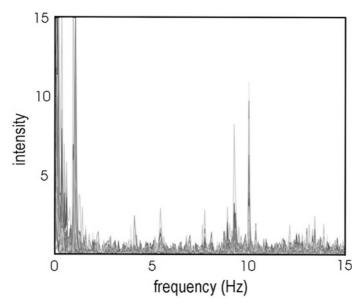
Fig. 4.1. Frequency spectrum of beam motion in the SLC linac, revealing the contribution of water pumps operating at 59 Hz [1]
