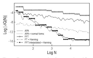
Fig. 2.6. Tune precision vs. number of turns, considering different FFT techniques applied to tracking data for the 4-D Hénon map [4]. The abbreviation 'APA' refers to a calculation of the average phase advance, which can be computed either in the original phase-space coordinates or in so-called normal-form coordinates. See [4] for more details on these alternative methods (Courtesy M. Giovannozzi, 1998)
