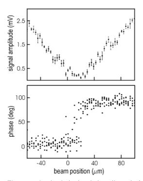
Fig. 3.10. Amplitude (top) and phase (bottom) of the beam-induced dipole mode signal in an X-band accelerating structure versus the nominal beam position (arbitrary zero), which was varied by steering correctors [16] (Courtesy M. Seidel, 1998)
