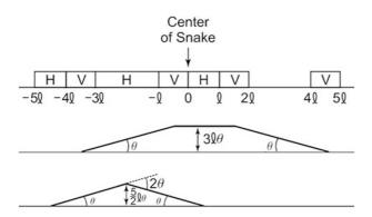
**Fig. 10.6.** A design of a type-1 siberian snake showing the geometry (top) and the design orbit in the vertical (middle) and horizontal (bottom) planes. The beam moves from the left to the right (Courtesy A. Chao, 1999)
