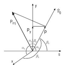
Fig. 10.2. Graphical representation showing the projection of the injected polarization  $P_{\rm inj}$  onto the stable spin direction  $\hat{n}_0$  at the injection point. The time-averaged vertical polarization one would measure at that point in denoted by  $P_y$
