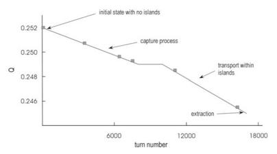
Fig. 9.18. Variation of the small-amplitude tune Q as a function of turn number n during resonant multiturn extraction [29]. The *solid squares* refer to tune values for which phase-space portraits are shown in Fig. 9.19 (Courtesy M. Giovannozzi, 2001)
