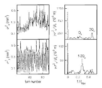
**Fig. 9.8.** Horizontal (top) and vertical (bottom) beam sizes for the first 100 turns after injection into the SLC damping ring (left) and their FFT (right) [18]. Clearly visible in the frequency spectra are lines at  $2Q_x$  (top) and at  $(1 - 2Q_y)$  (bottom), whose amplitude is a measure of the amount of beta mismatch
