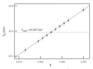
**Fig. 7.8.** Beam energy fitted from  $Q_s$  vs.  $\hat{V}$  measurement as a function of rf voltage calibration factor g; the *dotted line* indicates the known energy value, determined independently by resonant depolarization [15] (Courtesy A.-S. Müller, 2000)
