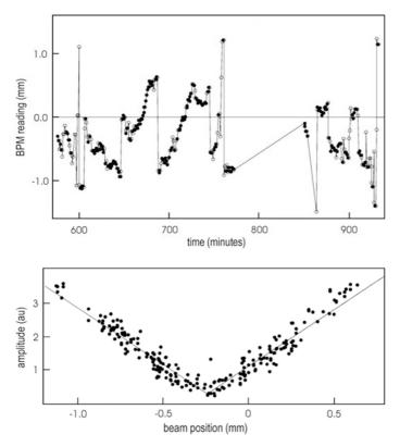
**Fig. 3.8.** Determination of BPM offsets using k modulation and natural orbit variation in LEP [6]: (top) natural orbit drifts and corrections during a LEP luminosity run at one quadrupole; (bottom) amplitude of beam response to k modulation vs. BPM orbit reading for the modulated quadrupole. The minimum of this plot gives the BPM offset. These data were taken continuously during 5 hours of luminosity run (Courtesy I. Reichel, 1998)
