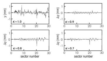
Fig. 3.20. Absolute and difference vertical trajectories measured after dispersion-free steering in the SLC linac (Courtesy R. Assmann, 2000)
