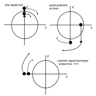
Fig. 11.10. Two-particle model of signal recoherence after applying first a dipole kick and then a quadrupole kick [45]. For the echo generation it is essential that the betatron tune depends on the oscillation amplitude
