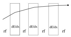
Fig. 11.17. Schematic of ionization cooling in the transverse phase space using a series of low-Z energy absorbers and reacceleration [52]
