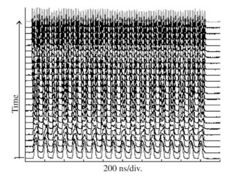
**Fig. 8.8.** Subsequent quadruple splitting at the CERN PS (E = 25 GeV,  $I_p = 8 \times 10^{12}$ , 1250 revolutions per trace). Compare with Fig. 8.5 (Courtesy R. Garoby, 2001)
