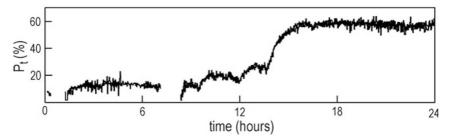
Fig. 10.4. Measured transverse beam polarization at HERA showing improvements gained using harmonic correction (Courtesy of the HERMES experiment, 2002)
