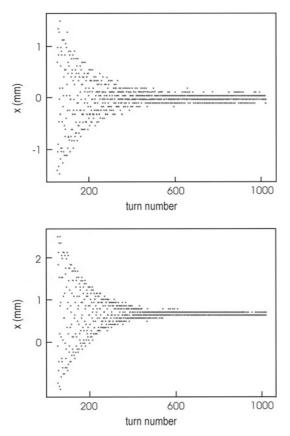
Fig. 2.4. Multi-turn orbit measurement for the motion of a single bunch in a train of 3 bunches at LEP-I. Shown are horizontal BPM orbit readings as a function of turn number: (top) BPM in a dispersive arc region; (bottom) BPM in a non-dispersive straight section. At the start of the measurement the bunch was deflected by a kicker. The corresponding FFT spectra are displayed in Fig. 2.5 (Courtesy A.-S. Müller, 2001)
