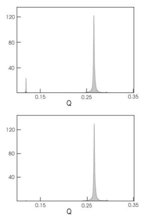
**Fig. 2.7.** Lomb normalized periodogram [12] for the two BPM measurements of Fig. 2.4 in a dispersive (*top*) and in a nondispersive region (*bottom*). The horizontal scale is in tune units, the vertical scale in arbitrary units (Courtesy A.-S. Müller, 2001)
