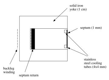
Fig. 9.15. Cross section of current sheet septum [6] (Courtesy M. Zisman, 2002)
