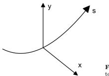
Fig. 1.1. Schematic of the reference trajectory and the transverse coordinate system
