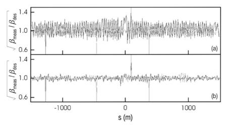
Fig. 2.14. Beta function measurement at KEKB, based on (2.36). Ratio of measured  $\beta$  function to the design value is shown before (*top*) and after optics correction (*bottom*) (Courtesy H. Koiso, 2000)
