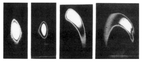
Fig. 4.13. Measured beam profiles demonstrating emittance growth due to wakefields as a function of increasing oscillation amplitude. From *left* to *right* the amplitudes in the applied horizontal trajectory displacement are 0 mm, 0.2 mm, 0.5 mm, and 1.0 mm. The single-bunch charge was  $2 \times 10^{10}$  electrons (Courtesy J. Seemann, 2000)
