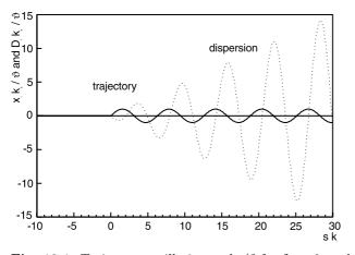
**Fig. 12.1.** Trajectory oscillation,  $x_1k_\beta/\theta$  for  $\delta_1 = 0$ , and resonantly growing dispersion at the bunch head,  $D_1k_\beta/\theta$ , induced by a deflection at s = 0, according to (12.21) and (12.22)
