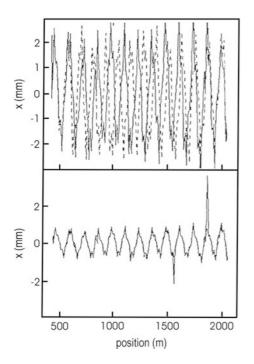
Fig. 3.15. Comparison of measured data and fit to betatron amplitude only (top) or fit to both betatron amplitude and energy in the different linac sections (bottom). Plotted is the horizontal beam position as a function of distance along the linear accelerator (Courtesy T. Himel, 1999)
