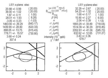
Fig. 4.3. Graphics output of multiple-wire transverse beam emittance measurement in the injector linac at the SLC
