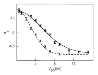
Fig. 10.5. Spin flip of a vertically polarized beam at the IUCF with kinetic energy 105.4 MeV and a frequency sweep range of 2 kHz. The estimated resonance strength at 15 kV applied voltage is  $1.9 \times 10^{-4}$  (Courtesy A. Krisch, 1999)
