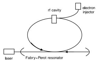
Fig. 11.9. Schematic of a laser-electron storage ring [31]
