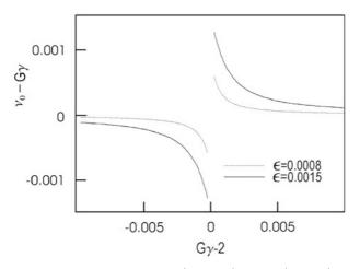
**Fig. 10.11.** Spin tune shift  $(\nu_0 - G\gamma)$  versus  $(G\gamma - 2)$  near an imperfection resonance, according to (10.58). The *dashed curve* corresponds to a resonance strength of magnitude 0.0008. The *solid curve* results for a resonance strength of 0.0015
