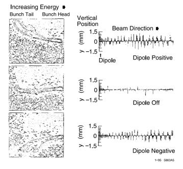
Fig. 4.12. Profile monitor measurements in a region of nonzero dispersion after the end of the SLC linac and vertical centroid trajectories with a positive purturbation to the bunch orbit (top), under nominal conditions (middle), and with a negative perturbation (bottom) (Courtesy J. Seeman, 2000)
