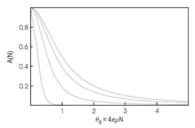
**Fig. 2.26.** Decoherence factor A(N) as a function of  $\theta = 4\pi\mu N$  for normalized kick strengths of Z = 0.2, 1, 2, and 5 (ordered from *top* to *bottom*)
