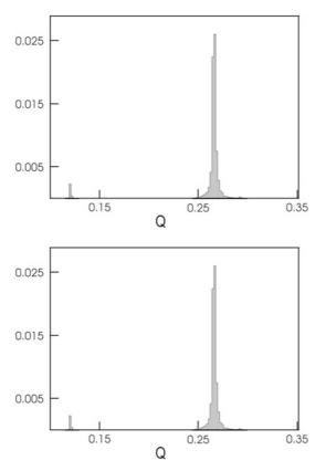
**Fig. 2.5.** FFT power spectra for the two BPM measurements of Fig. 2.4 in a dispersive (*top*) and in a nondispersive region (*bottom*). The horizontal scale is in tune units, the vertical scale in arbitrary units (Courtesy A.-S. Müller, 2001)
