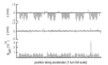
Fig. 7.2. Static dispersion measurement on the PEP-II HER: the orbit change induced by a 2 kHz shift in rf frequency. The nominal rf frequency is 476 MHz, the harmonic number h = 3492, and the momentum compaction factor  $\alpha_c \approx 0.0024$  (Courtesy U. Wienands, J. Seeman et al., 1998)
