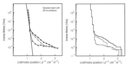
**Fig. 6.2.** Beam tails in LEP2 at 80.5 GeV: (*left*) measurement with collimation retracted (*circles*) and using movable scrapers at dispersive (*squares*) and nondispersive (*triangles*) locations, and (*right*) result of Monte-Carlo simulation [17, 18] (Courtesy H. Burkhardt, 1999)
