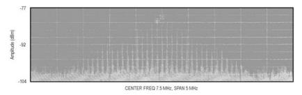
Fig. 7.1. Measurement of multiple synchrotron sidebands at injection in the SLAC electron damping ring. The synchrotron frequency is given by the difference in frequency between the fundamental and the nearest synchrotron sideband
