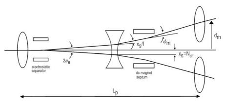
Fig. 9.20. Schematic of beam separation at the VLLC as described in [32]
