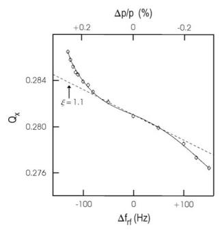
Fig. 7.12. Horizontal tune as a function of the change in rf frequency measured at LEP [21]. The *dashed line* shows the linear chromaticity as determined by the measurements at  $\Delta f_{\rm rf} = \pm 50$  kHz (Courtesy H. Burkhardt, 1998)
