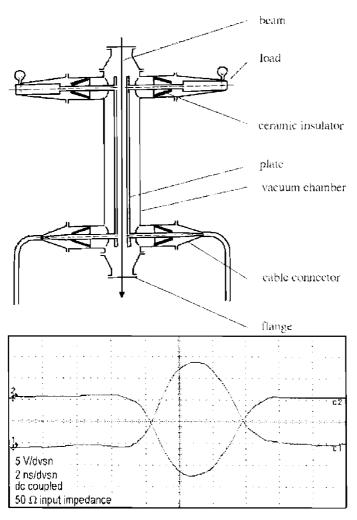
**Fig. 9.12.** Very fast kicker prototype [24]: (*top*) layout; (*bottom*) measured output rf pulses (Courtesy V. Shiltsev, 1998)
