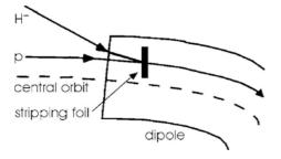
**Fig. 9.6.** Schematic of  $H^-$  stripping injection
