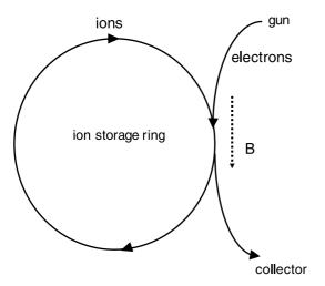
Fig. 11.1. Schematic of electron cooling for an ion storage ring
