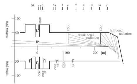
Fig. 6.3. Layout of the straight section around IP4 or IP8 in the horizontal and vertical planes. Shown are the quadrupoles (QS), electrostatic separators (ES), and collimators/masks (COLH, COLV, COLZ). The solid lines mark the inner vacuum chamber radii for the LEP1 layout [9, 21] (Courtesy H. Burkhardt, 1999)
