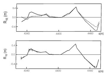
Fig. 2.17. Reconstructed R matrix element  $R_{16}$  in the SLC final focus from a sample of 100 simulated trajectories with fluctuations in betatron orbit and energy assuming a 20  $\mu$ m BPM resolution [33]: (top) standard  $\chi^2$  fit; (bottom) principal axes transformation. The fit results (dashed) are compared to the model used for the trajectory generation (solid) (Courtesy P. Emma, 1998)
