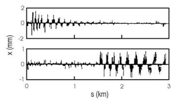
Fig. 4.14. Two trajectory ocillations in the SLAC linac, which were used to study the effect on the downstream emittance (Courtesy F.J. Decker, 1999)
