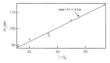
Fig. 7.9. Rms bunch length in the PEP-II HER as a function of the inverse synchrotron tune [18]. The fitted slope determines the momentum compaction factor  $\alpha_c$ , if the rms energy spread is known (Courtesy A. Fisher, 1998)
