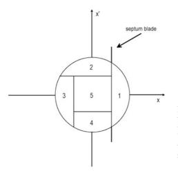
Fig. 9.17. Principle of the conventional 'continuous-transfer' extraction from the CERN PS ring. The beam is shaved by means of an electrostatic septum [29, 30]. The horizontal tune of the PS is set to 6.25 (Courtesy M. Giovannozzi, 2001)
