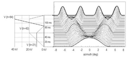
Fig. 8.5. Simulation of further bunch splitting in the CERN PS at high energy (26 GeV/c) in preparation for injection into the LHC. Compare with the measurements shown in Fig. 8.8 (Courtesy R. Garoby, 1999)
