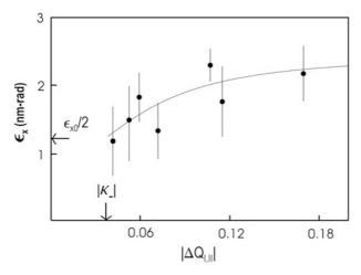
Fig. 2.31. Horizontal emittance as a function of the tune separation  $\Delta Q_{I,II}$  at the ATF Damping Ring; the measured data [77] as well as the result of a nonlinear fit to (2.90) are shown; the fitted coupling strength of  $|\kappa_{-}| \approx 0.037$  is consistent with the value  $|\kappa_{-}| \approx 0.042$  inferred from a simultaneous measurement of the closest tune approach [77, 71]
