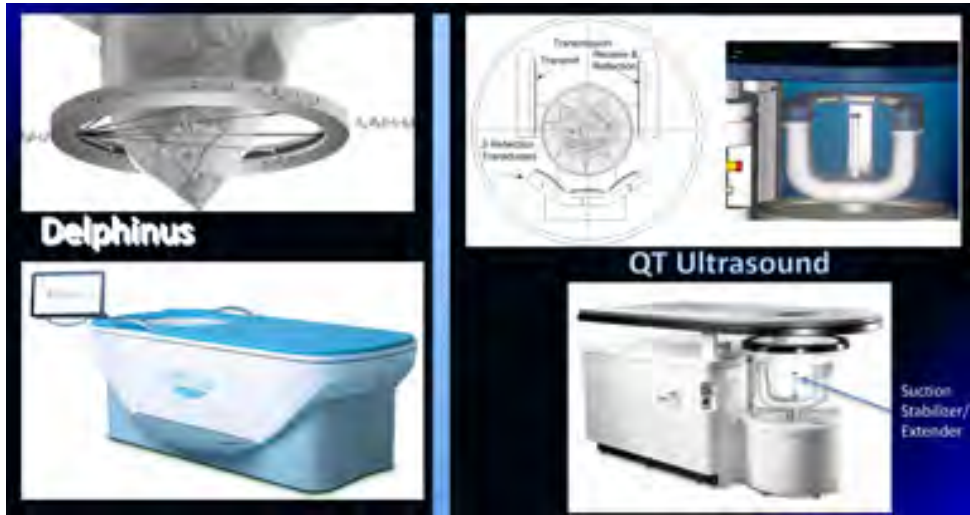
Figure 11: Two commercially available UTT systems. Left: Delphinus SoftVue [31] system with 2048 element ring array operating at up to 2.5 MHz; Right: QT Ultrasound’s system with a large, planar transmitter, a 1536 element transmitter and receiver array operating at 0.3 to 1.3 MHz and three conventional curved linear arrays conventional pulse echo imaging [32].
