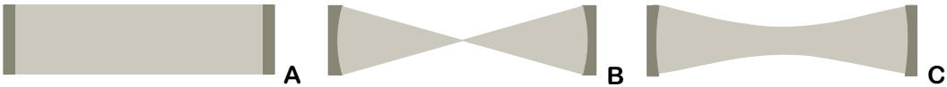
FIGURE 10.31 Examples of optical cavities. Plane-parallel (A), concentric/spherical (B) and confocal (C) configurations.
