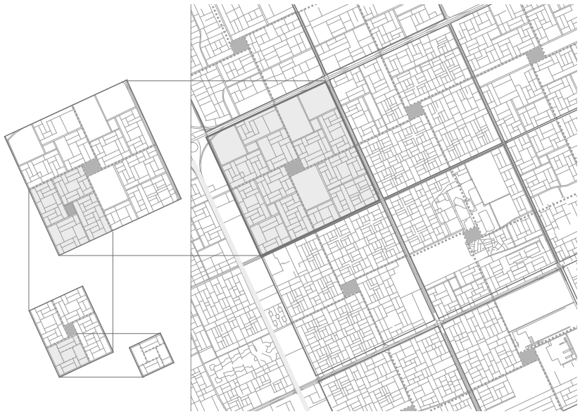
fig.5 1972 masterplan. Right: detail of the two-by-two km grid. Left: growth mechanism of the superblock (Source: Faisal Al-Mogren, 2020. Reuse not permitted)
