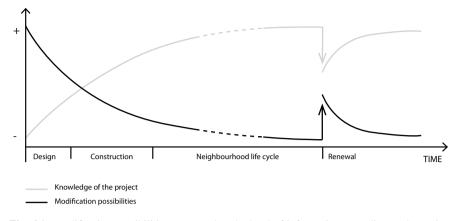
Fig. 6.1 Modification possibilities compared to the level of information according to the project progress
